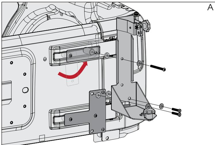
**If no Rugged Ridge tire carrier is present**, rotate Upper Mounting Plate into horizontal position and tighten upper left tailgate hinge bolt to hold in place. If using with Hard Top, add M8 spacer between Mounting Plate and Jack Mount.
