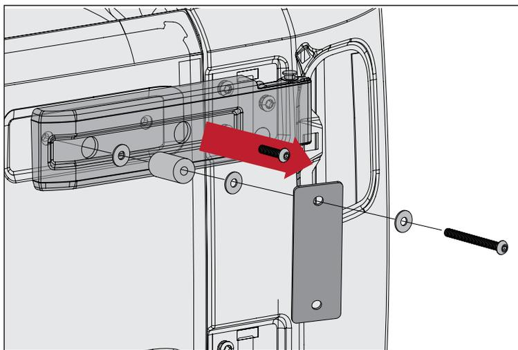
4. Install Lower Mounting Plate by first removing two lower tailgate hinge bolts. Attach lower hinge cover and use M8 hardware and spacers to secure Lower Mounting Plate to tailgate.
